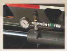
**Pressure Gauge and Sensor** Each hydraulic steering line has its own pressure gauge and sensor.
