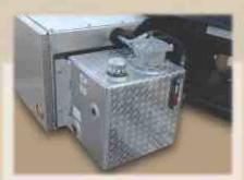
**Aluminum Hydraulic Oil Reservoir** Includes high micron filter for clean fluid, oil level sight gauge, and thermometer.
