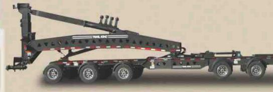
**Dolly Self-Contained Hydraulic**s 13 H.P. Honda self-contained hydraulic unit provides power to rear gooseneck at ground level.
