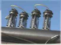
**Multi-Position Air Locks**Air locks on the tower lift link allow the operator to set tower ride height from ground level.
