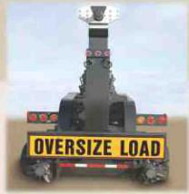
**Telescoping Mast**Works with tower flange inner diameter from 119" to 169" and maximum flange thickness up to 6".
