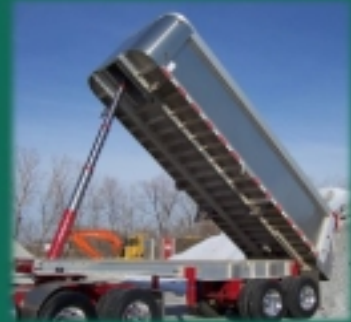
Frame Type Aluminum Dump Trailer (Steel Frame is Standard; Aluminum Frame is Optional)
