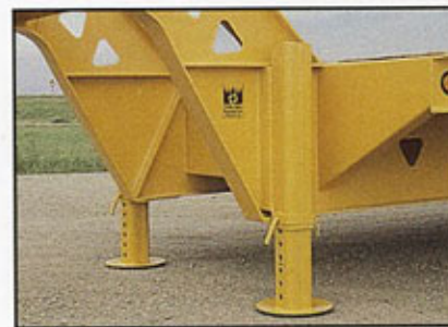
Telescopic pin-type park stands are standard. A two-speed landing gear is offered as an option.
