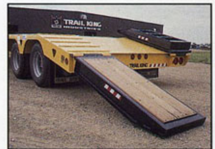
Optional wood-filled crawler ramps can be added to the standard 30" beavertail for ease of loading.
