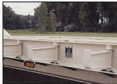
Heavy duty swing-out outriggers are optional for hauling extra-wide loads. D-rings on 48" centers are standard.
