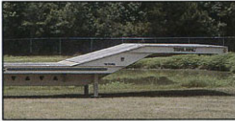
Trailer as shown features a full upper deck with a special 15 degree slope for extra ease in loading the upper deck.
