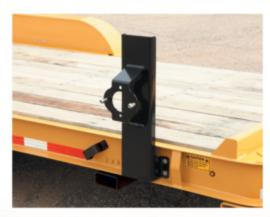
**Bolt-On Spare Tire Carrier**An available option that allows you to safely mount and easily remove a spare tire.
