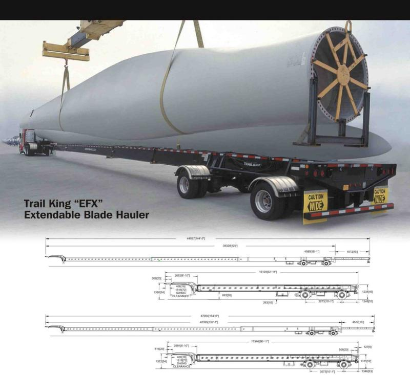
The EFX Extendable is designed to accommodate a variety of blade sizes and styles. Its narrow, double-telescopic, monoframe main frame can haul two blades at one time and, together with a low profile gooseneck, keeps overall dimensions to a minimum. And, with hydraulic turntable-style steering, these long loads can be maneuvered with ease while in transit or at the job site.
