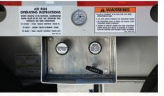
**Air Ride Suspension Controls** The air control panel is housed in an aluminum control box conveniently located between the axles on the driver's side of the trailer. No more having to climb up on the trailer or reach over a flip axle to get to the controls.
