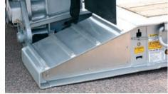
Extended Tapered Front Approach The front approach ramps, featuring heavy duty 3/4" full-width traction aids, have been extended forward to lower the front edge of the ramp to only 4". Ramp pullouts can be added by simply removing the aluminum side panels.
