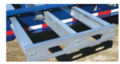
OPTIONAL **Aluminum Pull-Out Outriggers** Aluminum pull-outs include full-width aluminum box beam cross members on 16' centers. The pull-outs, when fully extended, provide an overall trailer width of 13 feet.
