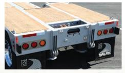
**New Wheel Area Tail Channel** The wheel area is standard with steel outer rails, crossmembers, and tail channel, as well as dock bumpers, and flip axle reinforcements. (Exception: flip axle reinforcement is an add-on option on the TK70MG-HG model.)
