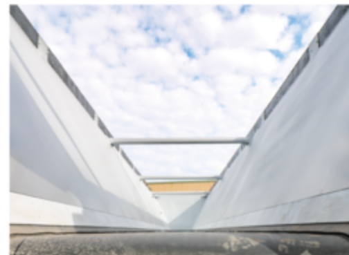
Hopper Walls Constructed with longer lasting .160" (4mm) thick AR450 wear plate (rear half standard, full length optional).
