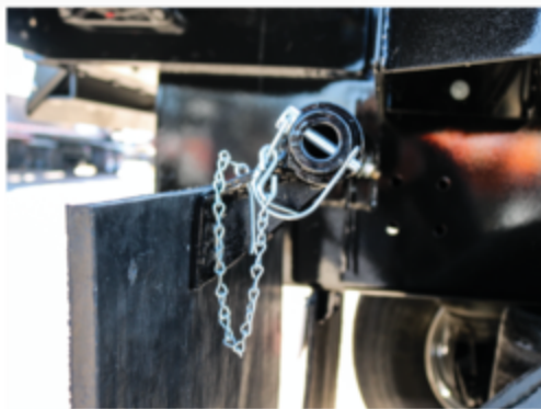
Flip-Up Mud Flaps Convenient hinged design for better paver hopper clearance. Optional auto flip-up.
