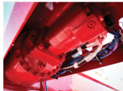
Hydrostatic Drive Single or dual direct hydrostatic drive w/ double reduction planetary gearbox and drive tube.
