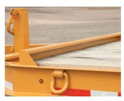
**Safety Headboard** The safety headboard provides extra dimension of safety and load-hauling security.
