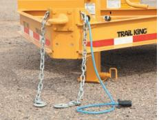
**Adjustable Hitch** Accommodate a wide variety of towing vehicles with an adjustable 4-bolt hitch rated for the full GVWR of the trailer.
