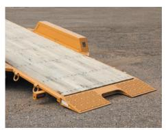
**Approach Plate** The main deck tilts to an 11° load angle, and features star traction material on the approach plate and recessed lights that are protected during the loading/unloading process.
