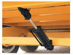
**Platform Cushioning Cylinders** Single platform cushioning cylinders make loading and unloading a smooth operation.
