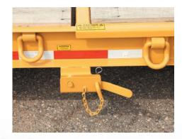
**Platform Lock** Keep your deck from accidentally tilting while in the transport mode with the platform lock mechanism and safety lock pin.
