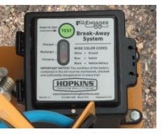
**Break-Away System** The lighted read-out break-away system monitor provides easy and convenient monitoring of the charge status.
