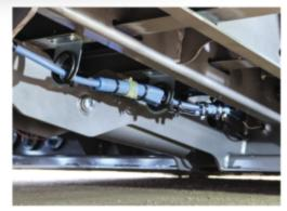
**Ground Clearance**Flip tail linkage bracket and pin have increased ground clearance in loading position.
