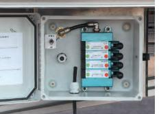
**Air-Operated Control Valves** High guality air-operated valves are contained in a conveniently located, protective sealed box, and control the slider axle brakes/locks and suspension raise/lower functions. Actual functions will vary based on trailer options.
