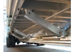
**Floating Knee Braces and** Aluminum Crossmembers Knee braces are bolted on, not welded, reducing stress on the main beam and crossmembers. Crossmembers are on 12" centers in the main deck and 18"
