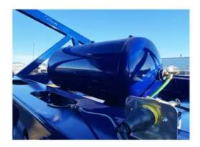
Large Air Reservoir Standard 60 gallon air reservoir allows more capacity for the gate and quicker operation.
