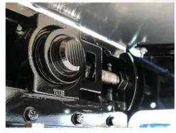
Front Bearing Assembly Heavy duty outboard design for easier maintenance.
