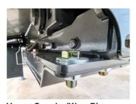
**Upper Coupler/King Pin**Bolt-on design allows for simpler maintenance and better access.
